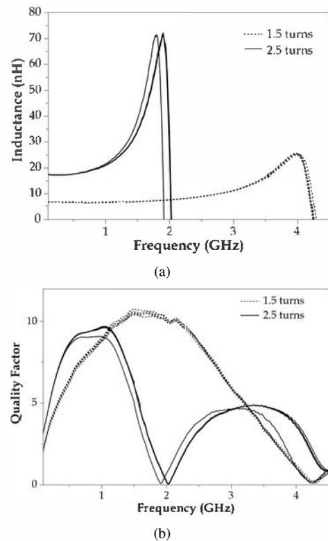
Fig. 4. Performance of the 1.5 turns (dashed lines) and 2.5 turns (solid lines) inkjet printed inductors deposited on photographic paper.
