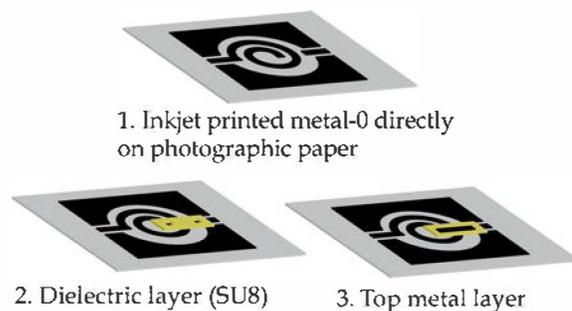
Fig. 1. Schematic example of multi-layer inkjet printing process.
