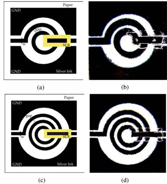
Fig. 3. Inkjet printed 1.5 turns and 2.5 turns MIM inductors: (a-c) design top view and (b-d) photographs of the respective prototypes.
