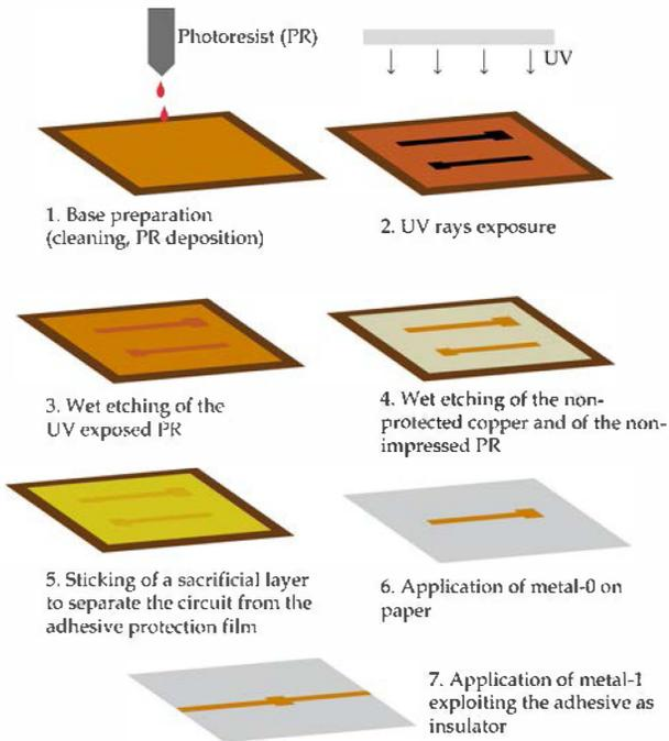
Fig. 2. Step-by-step illustration of the copper laminate method.
