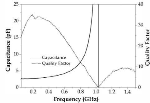
Fig. 6. Copper laminate capacitors on cellulose substrate: performance in terms of  $C$  and  $Q$ . The maximum  $Q$  is 22 and the SRF is 1 GHz.
