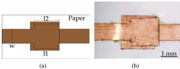
Fig. 5. Copper laminate capacitors on cellulose substrates: (a) top view of the geometry and (b) micrograph of the prototype.
