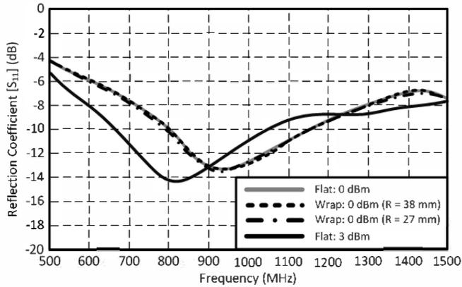
Fig. 4. Measured reflection coefficient values ( $S_{11}$ ) of the designed RF-DC converter.
