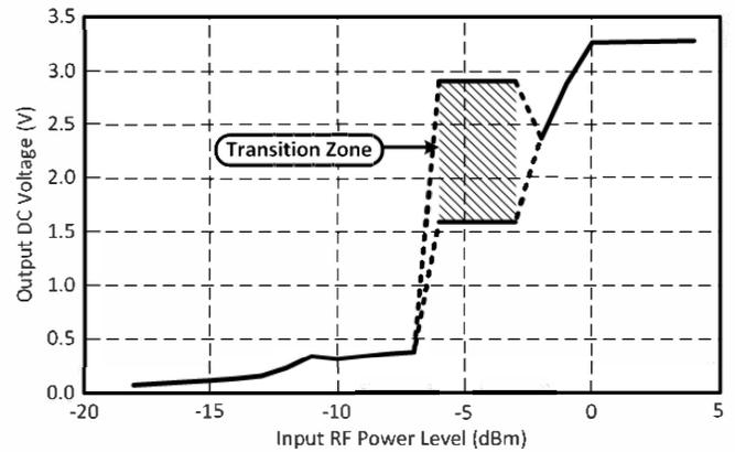
Fig. 5. Measured output DC voltage depending on input RF power level: flat and bent circuit at 900 MHz.
