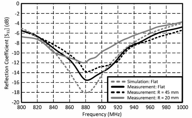
Fig. 3. Measured reflection coefficient values ( $S_{11}$ ) of the flexible square loop antenna.
