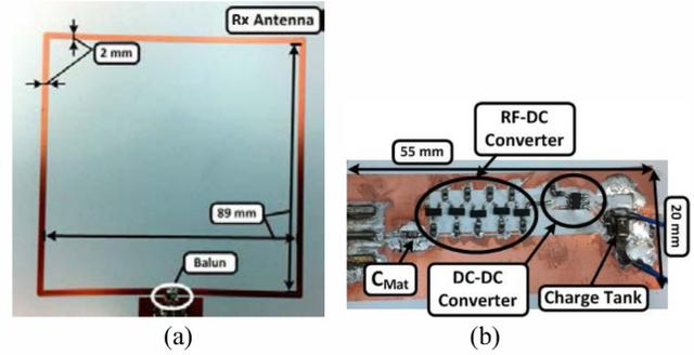
Fig. 2. Hybrid printed flexible RF energy harvester on a low-cost polymer: (a) square loop antenna, (b) RF-DC converter.
