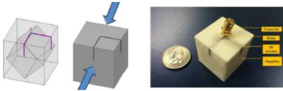
Fig 7. 3D printed strain sensor with embedded cavity
