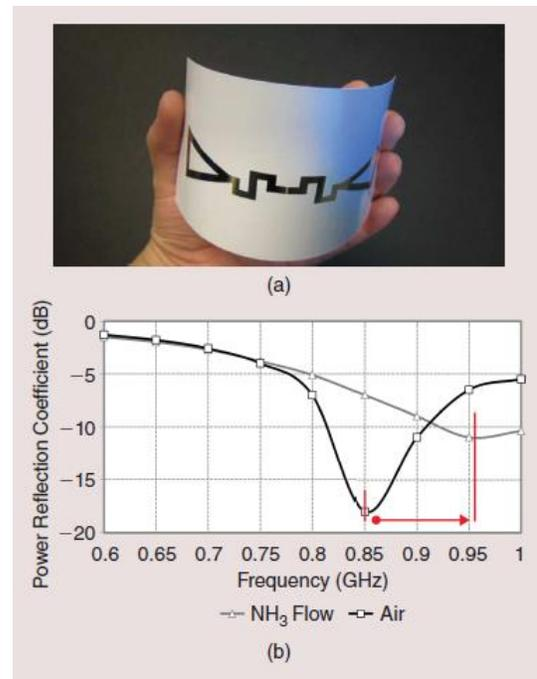
Fig 1. Inkjet-printed CNT-based wireless sensor.
