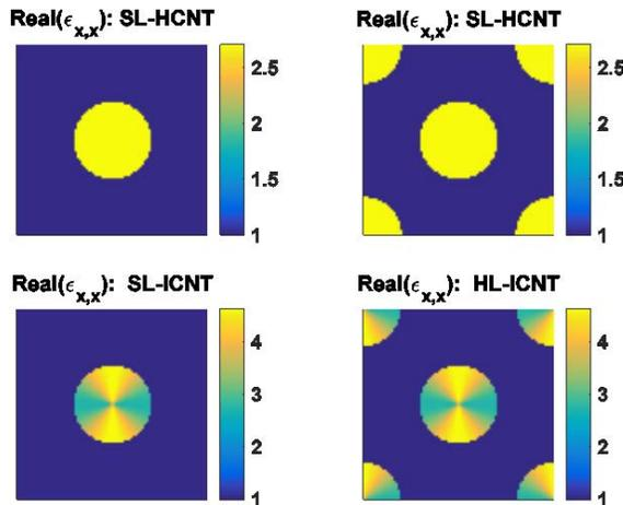
Fig 2. Lattice arrangement of CNT’s: SL-HCNT: Square Lattice Homogeneous CNT, SL-ICNT: Square Lattice Inhomogeneous CNT, HL-HCNT: Hexagonal Lattice Homogeneous CNT, HL-ICNT: Hexagonal Lattice Inhomogeneous CNT (only the  $\epsilon_{x,x}$  permittivity tensor element is shown).
