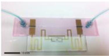
Fig 4. (a) Inkjet-printed liquid-reconfigurable wireless sensor.
