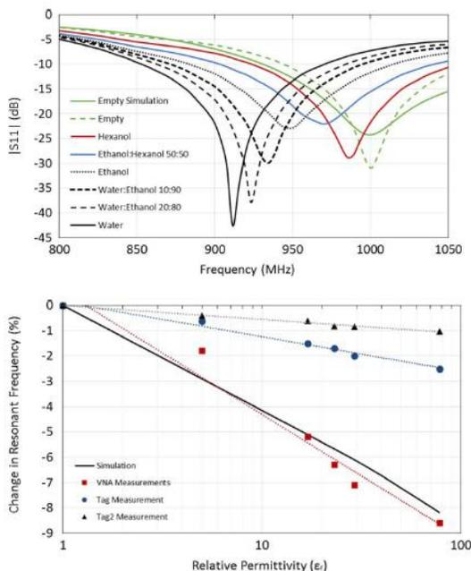
Fig 4. (b) Liquid-based reconfigurability/sensitivity
