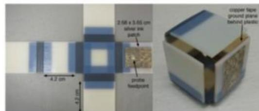
Fig 6. 4D printed "morphing" energy harvesting cuboid
