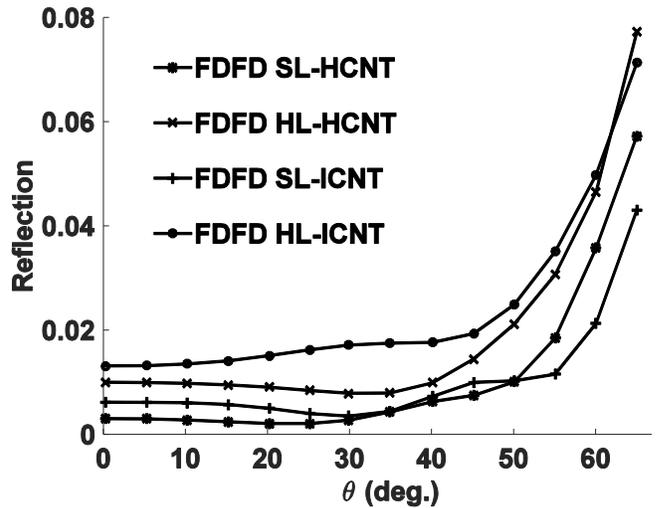
Fig 3. Reflection coefficient of the CNT lattice arrangements of Fig. 2, as a function of the polar angle  $\theta$  of the incident plane wave. Design parameters: Incident Wavelength:  $0.5\mu\text{m}$ , Tube Diameter:  $80\text{nm}$ , Unit Cell Size (in  $x, y$  directions):  $0.2\mu\text{m}$ , Tube Length:  $1\mu\text{m}$ .
