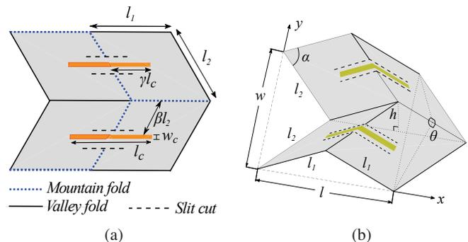
Fig. 1: Unit cell of Miura FSS in (a) flat state ( $\theta = 180^\circ$ ) (b) folded state with  $l_1 = l_2 = 20mm$ ,  $\alpha = 45^\circ$ ,  $\beta = \gamma = 0.5$ ,  $l_c = 20mm$  and  $w_c = 2mm$ .
