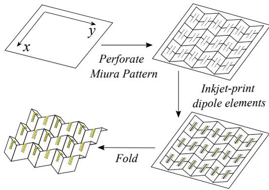
Fig. 2: Fabrication process for single-layer Miura FSS.
