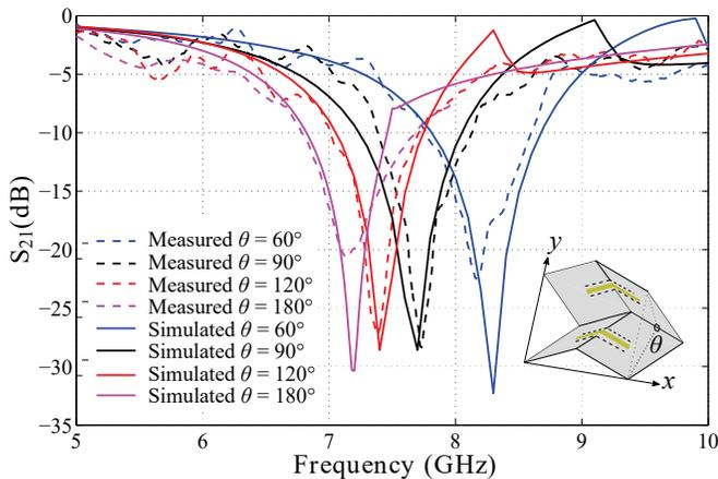
Fig. 5: Frequency response of single-layer Miura-FSS with different values of folding angle  $\theta$ .
