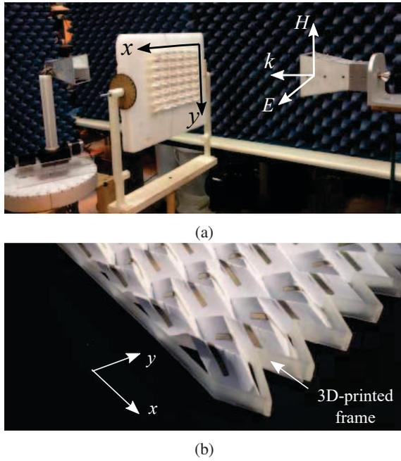
Fig. 4: (a) Measurement setup (b) 3D-printed frame to uniformly fold Miura-FSS structure at a given folding angle  $\theta$  (frame for  $\theta = 90^\circ$  is shown here).
