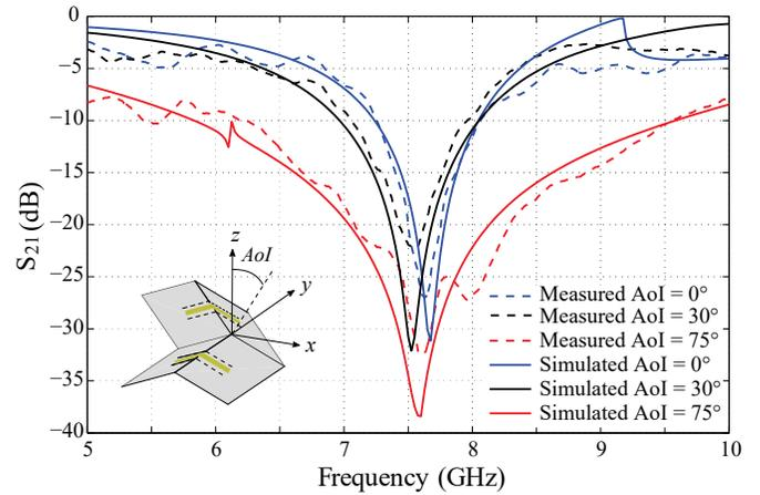
Fig. 6: Frequency response of single-layer folded ( $\theta = 90^\circ$ ) Miura-FSS with different values of angle of incidence.
