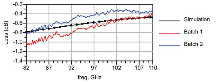
Fig. 2. Probe-station measurements of 1 mm-long CPW structure along with predicted performance of inkjet-printed silver lines on LCP.
