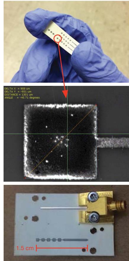
Fig. 1. Top: Inkjet-printed W-band array prototypes. Center: Microphotograph of W-band array patch element. Bottom: 1.0-mm top-launch connector attached to prototype's calibration line.
