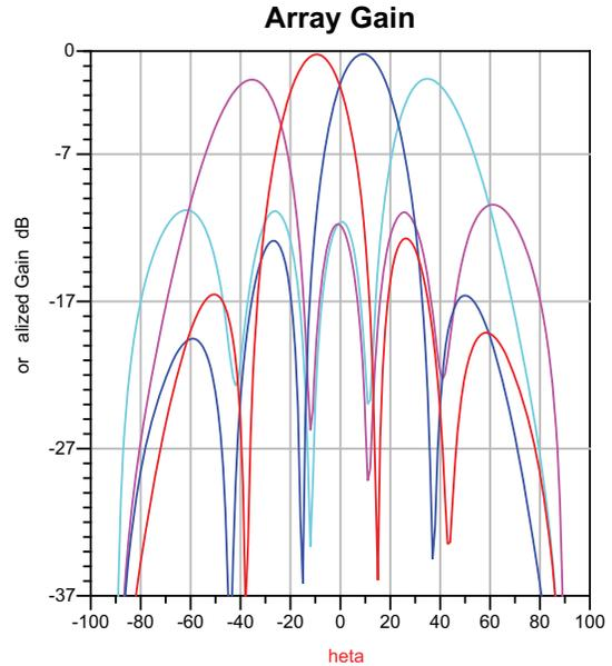
Fig. 6. Expected  $4 \times 5$  array gain with Butler matrix excitation.
