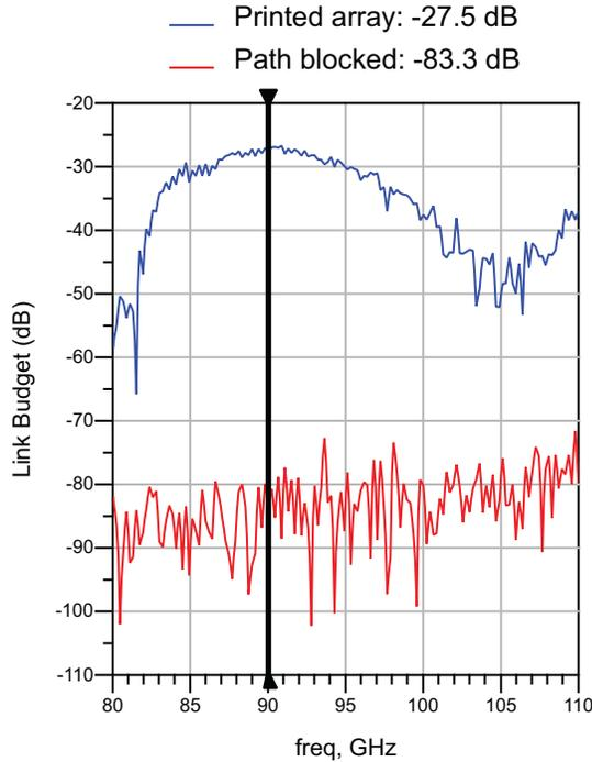
Fig. 4. Top: wireless measurement setup using W-band frequency extenders. Bottom: Link budget measurement with inkjet-printed array and reference WR-10 horn.
