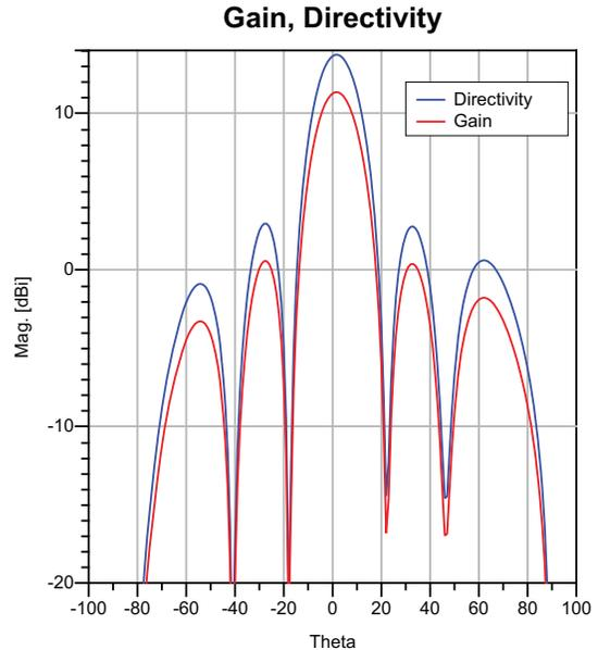
Fig. 3. 1  $\times$  5 printed W-band array directivity and realized gain at 90 GHz.
