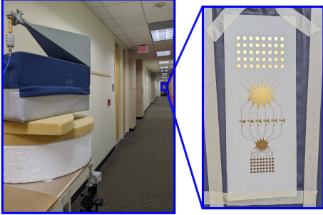
Fig. 5. Experimental setup for long-range demonstration of a proof-of-concept fully passive lens-enabled mmID at 65 m.
