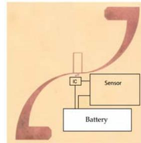
Figure 7. (a) Block diagram of RFID/Sensors tag (b) Suggested outline of integrated S-shaped antenna with IC, sensor and embedded battery.
