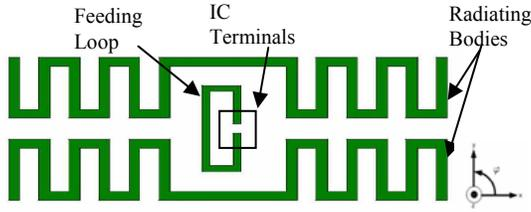
Figure 3. Dual Radiating body configuration
