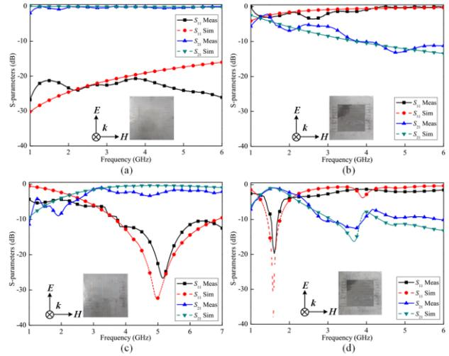
Fig. 5. Comparison of measured and simulated scattering parameters of the proposed FSS structure for different working states. (a) Both channels are empty, (b) top channel is filled with EGaIn, (c) bottom channel is filled with EGaIn, and (d) both channels are filled with EGaIn.
