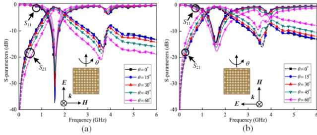
Fig. 3. Simulated scattering parameters of the proposed FSS structure (when both channels are filled with EGaIn) for various incident angles under (a)  $y$ - and (b)  $x$ -polarized incident wave. The solid and dotted lines represent the reflection and transmission coefficients, respectively.
