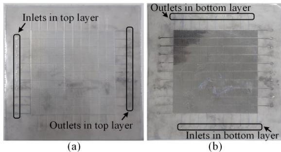
Fig. 4. Photographs of the fabricated prototype. (a) Before and (b) after the injection of EGaIn in both microchannels.
