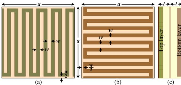
Fig. 1. Unit cell geometry of the proposed AFSS. (a) Top view of top layer, (b) top view of bottom layer, and (c) side view. Geometric dimensions are optimized as follows:  $a = 10$  mm,  $w = 0.5$  mm, and  $t = 1$  mm.
