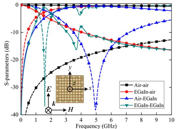
Fig. 2. Simulated scattering parameters of the proposed multifunctional FSS structure for different working states under  $y$ -polarized incident EM wave.
