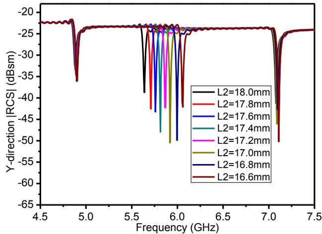
Fig. 3. Simulated RCS magnitude of the proposed tag in the Y direction with a Y-polarized incident wave corresponding to different length of  $L2$ .
