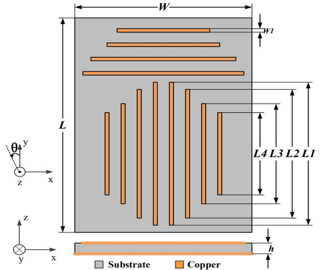
Fig. 1. Geometry of the proposed sensor tag. Dimensions are  $L = 30 \text{ mm}$ ,  $W = 22 \text{ mm}$ ,  $L1 = 20 \text{ mm}$ ,  $L2 = 18 \text{ mm}$ ,  $L3 = 14 \text{ mm}$ ,  $L4 = 11.5 \text{ mm}$ ,  $W1 = 0.5 \text{ mm}$ , and  $h = 0.8 \text{ mm}$ .
