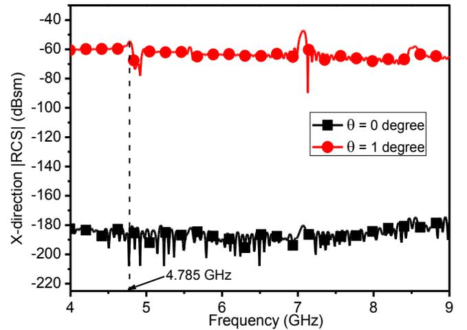
Fig. 4. Simulated RCS magnitude in the X direction when the rotation angle  $\theta$  is 0 degree and 1 degree, respectively.
