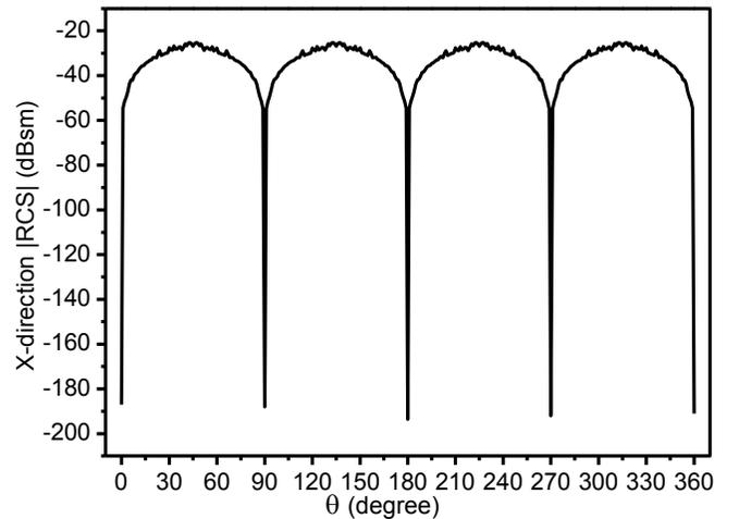
Fig. 5. Simulated RCS magnitude in the X direction at 4.785GHz when  $\theta$  varies from 0 degree to 360 degrees.
