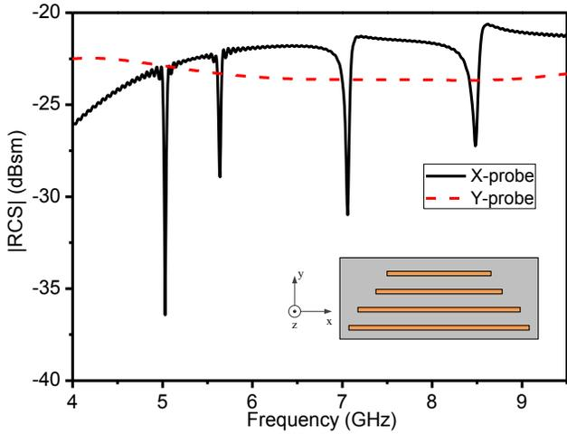
Fig. 2. Simulated RCS magnitude of the independent horizontal part of the proposed tag corresponding to X- and Y- polarized incident waves.
