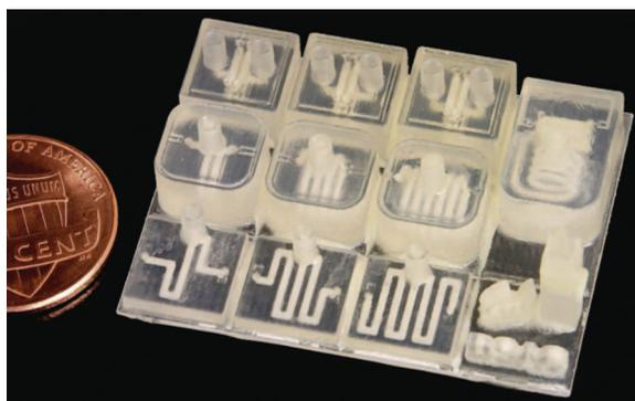
**Figure 1.** Several 3-D-printed passive components using material jetting. From top row to bottom: a capacitor, inductor, and resistor of various values [13].
