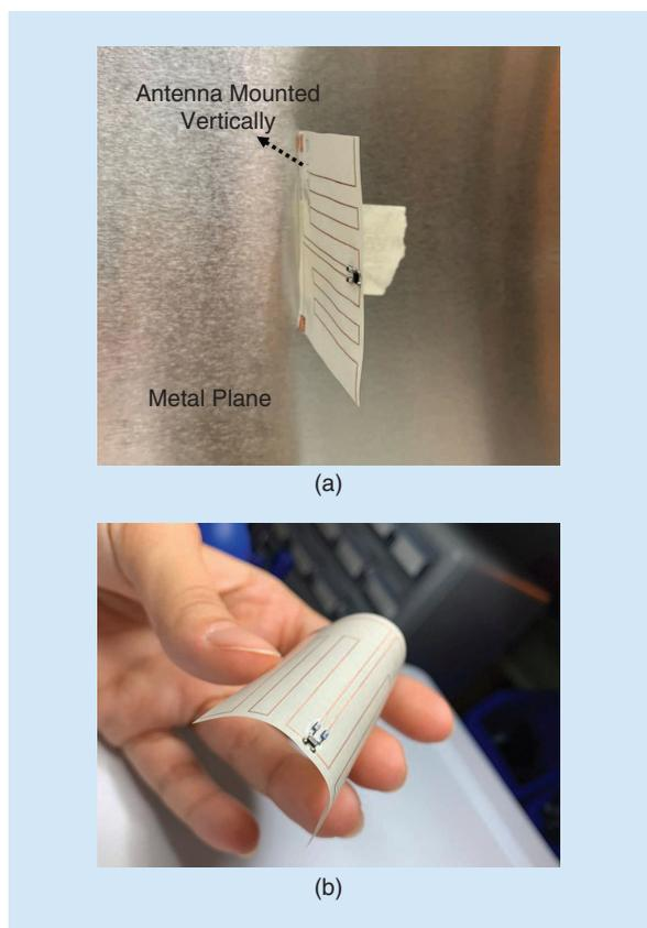
**Figure 6.** (a) The mounted backscatter modulator. (b) A profile of the assembled backscatter modulator showing its flexibility.
