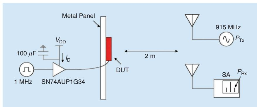
**Figure 1.** A diagram showing the measurement setup. DUT: device under test;  $V_{DD}$ : voltage drain drain;  $I_D$ : drain current; SA: spectrum analyzer.
