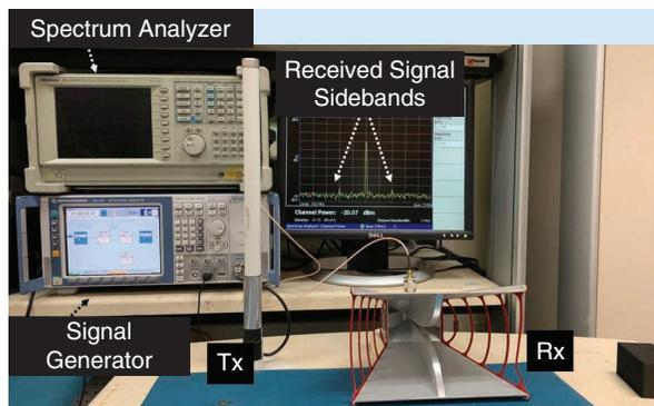
**Figure 5.** The laboratory setup. Tx: transmitter; Rx: receiver.
