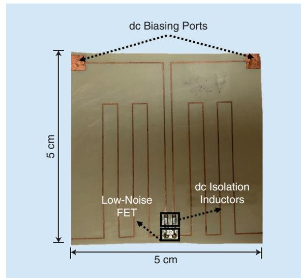
**Figure 4.** The assembled backscatter modulator.
