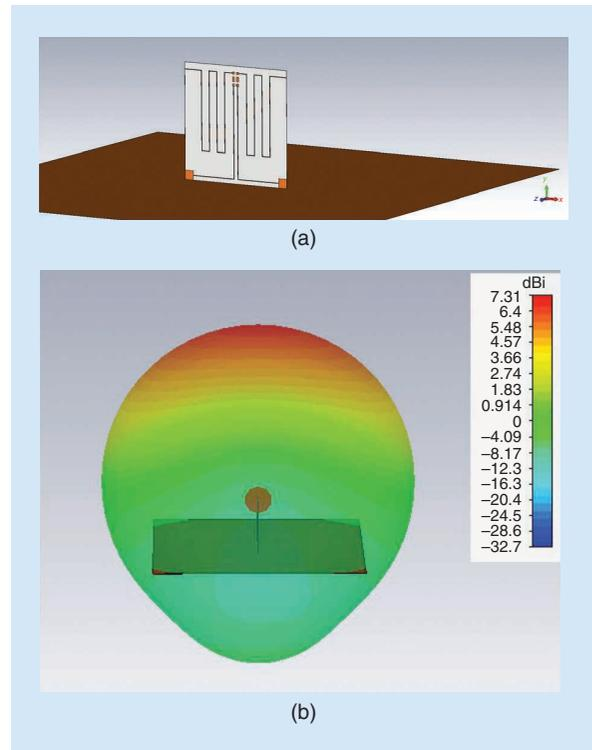
**Figure 3.** (a) An illustration showing a simulation model (using CST Microwave Studio 3D electromagnetic simulation software) of an antenna perpendicular to a metal sheet. (b) A simulated radiation pattern (gain: 7.313 dBi).
