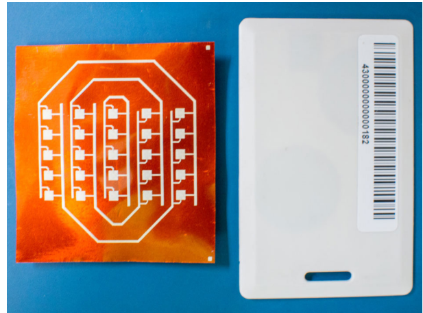
Fig. 2. Inkjet-printed flexible Van Atta reflectarray prototype, next to a standard “credit card” size RFID tag package [21].
