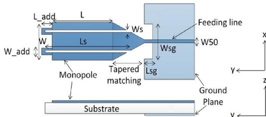
Fig. 7. The geometry of the proposed broadband planar monopole antenna.
