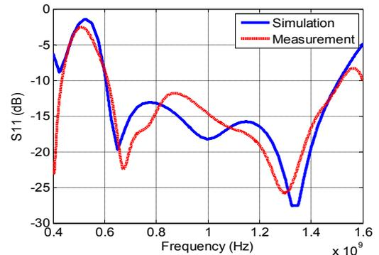
Fig. 8. The simulation and measurement results of  $S_{11}$  for the proposed antenna.
