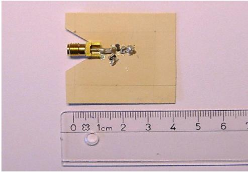
Fig. 5. The fabricated rectifier using inkjet printing technology on cardboard.
