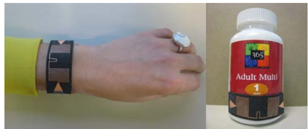
Fig. 2. Embodiments of the conformal RFID tag prototype in the applications of wireless health monitoring and pharmaceutical drug bottle tracking.
