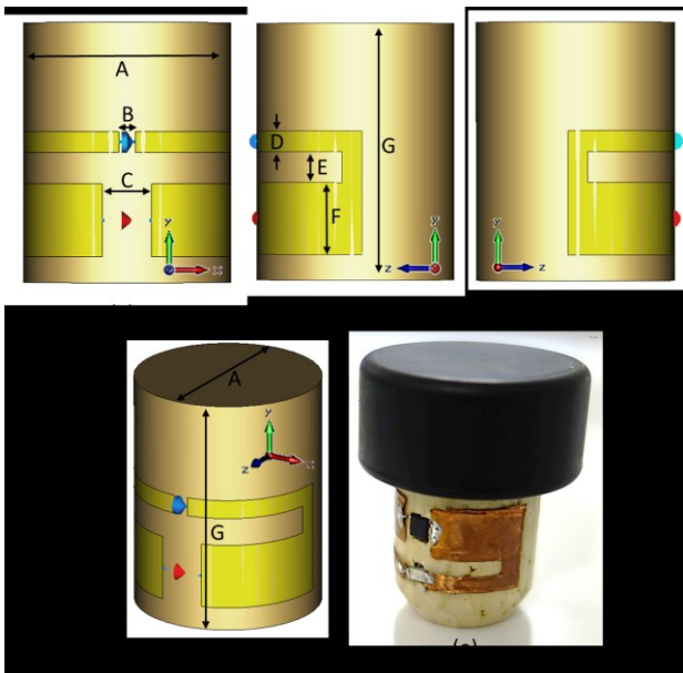
Fig. 3: Implementing an antenna in cork.
