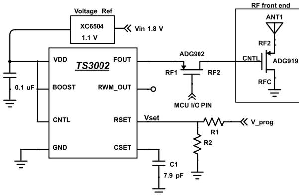
Fig. 5. Timer and RF front-end schematic of the tag. The timer produces square wave pulses with 50% duty circle and supplies the RF front-end through a modulation switch (ADG902). The ADG902 switch is controlled by the MCU.
