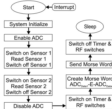
Fig. 9. Flow chart of the tag algorithm. This algorithm was implemented in the MCU and controls all the peripherals of the tag.
