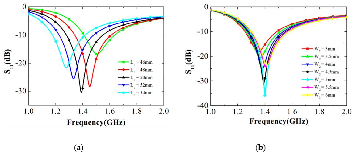
**Figure 2.** Simulated S-parameters of the proposed loop antenna at different parameters of (a)  $L_1$  and (b)  $W_2$  in the unfolded state.
