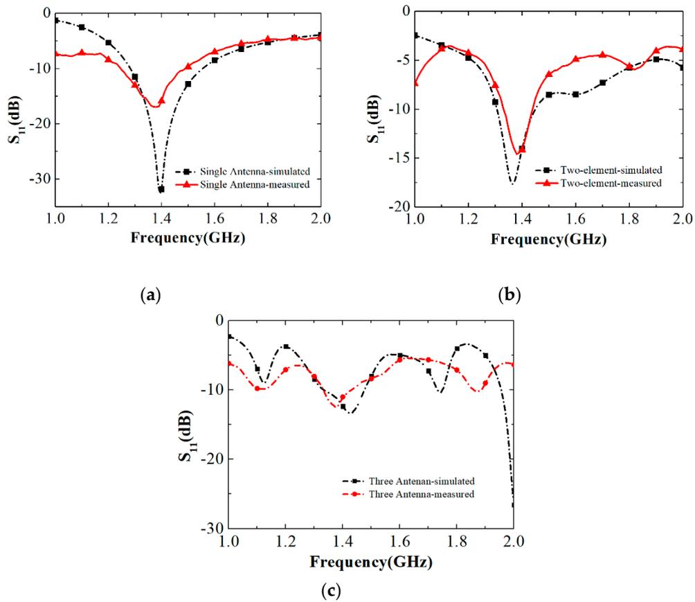
**Figure 7.** Simulated and measured  $S_{11}$  for (a) the single antenna, (b) two-element antenna array, and (c) three-element antenna array.
