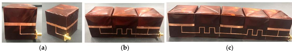
**Figure 6.** Fabricated samples: (a) Single antenna element, (b) two-element antenna array and (c) three-element antenna array.
