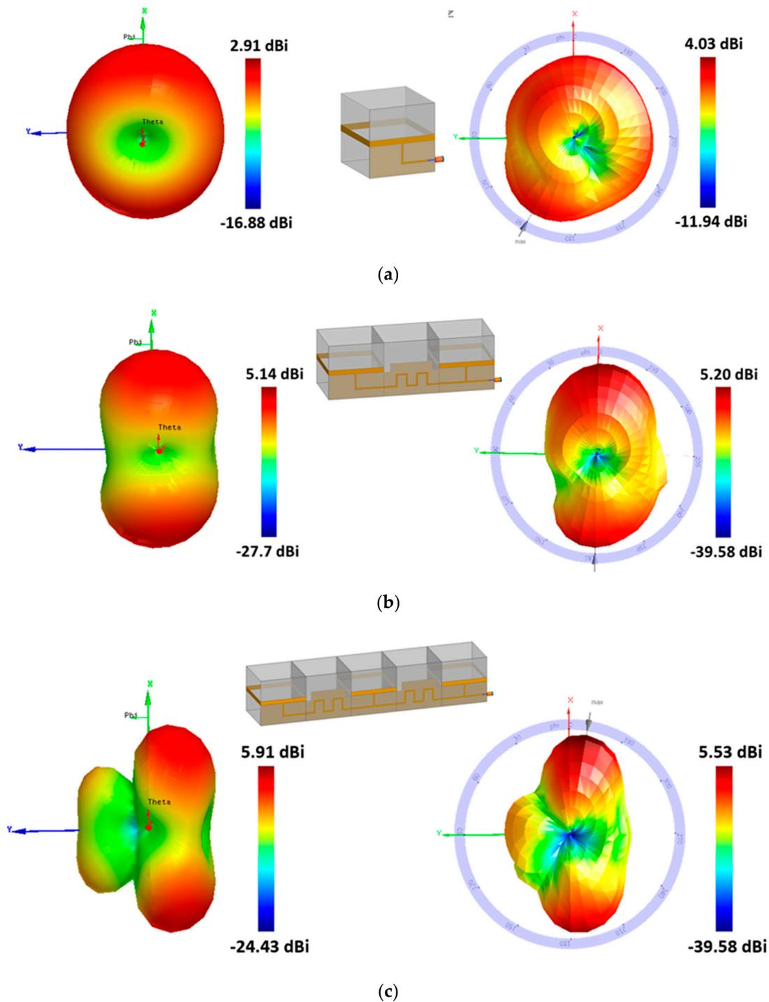
**Figure 8.** Simulated and measured 3D radiation patterns at 1.39 GHz for (a) the single antenna and (b) two-element antenna array and (c) three-element antenna array.
