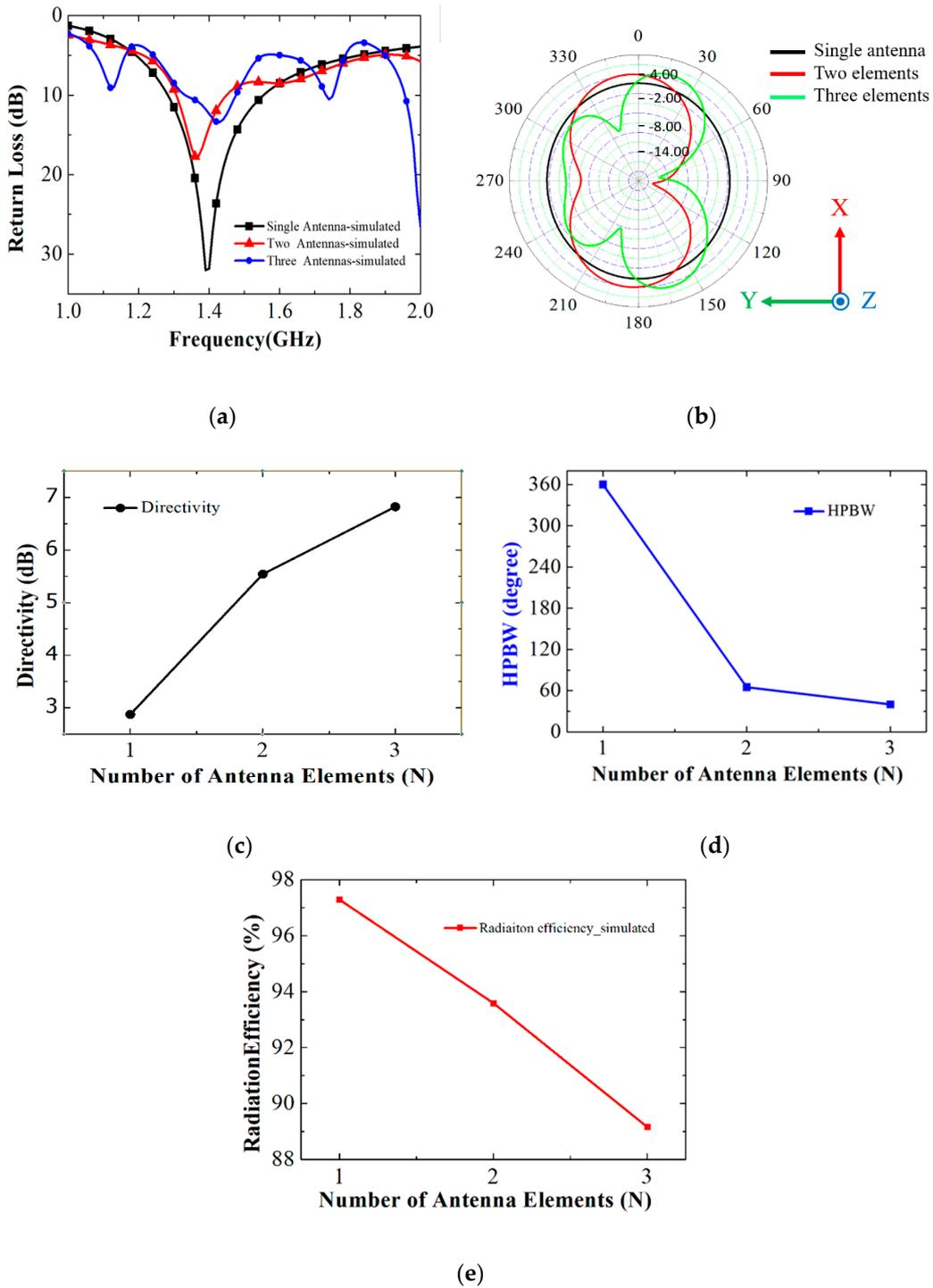
**Figure 4.** Simulated (a) return loss, (b) 2D radiation pattern on XY plane, (c) directivity, (d) half-power beam width (HPBW), and (e) radiation efficiency for different numbers of antenna elements of the antenna array.
