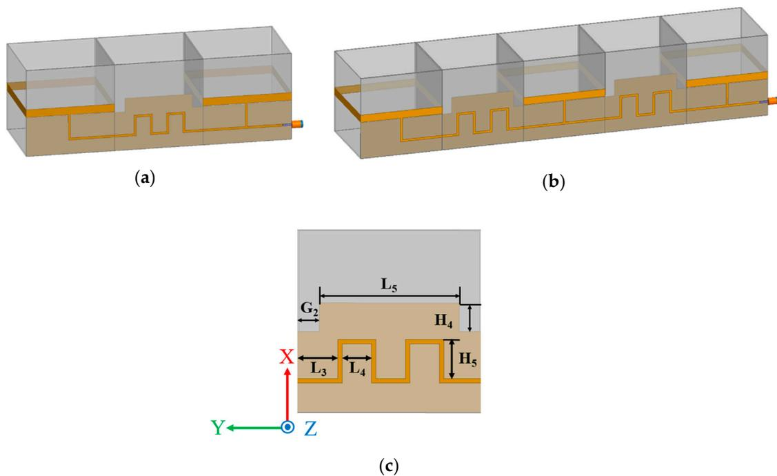
**Figure 3.** Illustration of the (a) two-element antenna array and (b) three-element antenna array. (c) Layout of the series feeding line.
