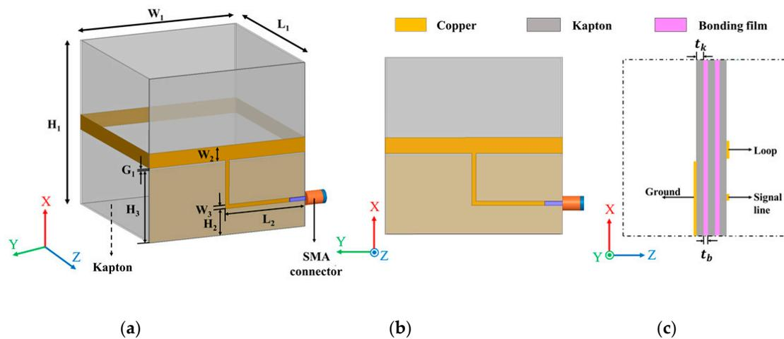
**Figure 1.** Illustration of the single magic cube antenna: (a) Angled view, (b) front view, and (c) overlapping layers at  $z = L_1$  and  $y = W_1$ .
