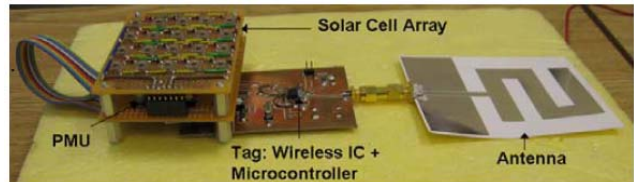
Fig. 8. Working solar powered end node prototype.
