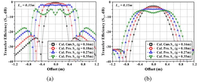
Fig. 9. PTE with regard to the offset between the transmitting and receiving antennas at different TX spacings ( $g$ ). (a)  $h_1 = 0.25$  m. (b)  $h_2 = 0.5$  m.
