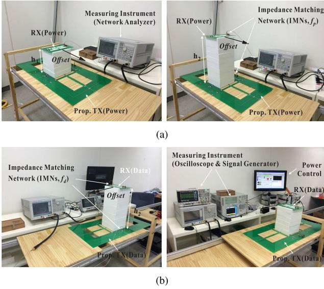
Fig. 13. Measurement setups of transfer efficiency ( $S_{21}$ ) with regard to a misalignment at the operating distance ( $h_1$  and  $h_2$ ) using measuring instruments. (a) Power transfer link. (b) Data communications link.
