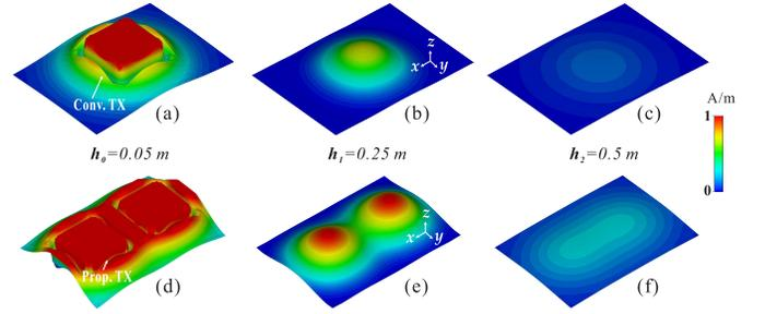
Fig. 7. Magnetic field distributions with regard to different air gaps ( $h$ ) away from the TX antennas for power transfer.
