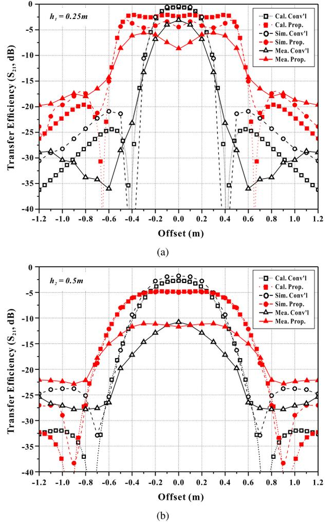
Fig. 14. Power transfer efficiency comparisons among the calculated, simulated, and measured results regarding the offset between the transmitting (conventional or proposed) and receiving antennas at different operating distances ( $h$ ). (a)  $h_1 = 0.25$  m. (b)  $h_2 = 0.5$  m.
