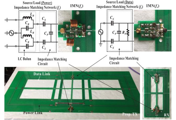
Fig. 11. Fabricated prototype and IMN schematics in the power and data links.
