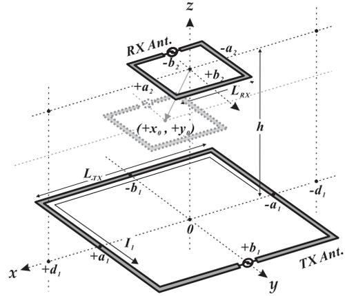
Fig. 5. Mutual inductance between two single loops with a misalignment.
