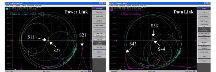
Fig. 12. Measured input impedance on Smith chart at the distance ( $h_2$ ).
