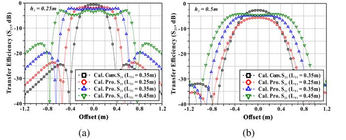
Fig. 8. PTE with regard to the offset between the transmitting and receiving antennas at different TX antenna lengths ( $L_{T1}$ ). (a)  $h_1 = 0.25$  m. (b)  $h_2 = 0.5$  m.
