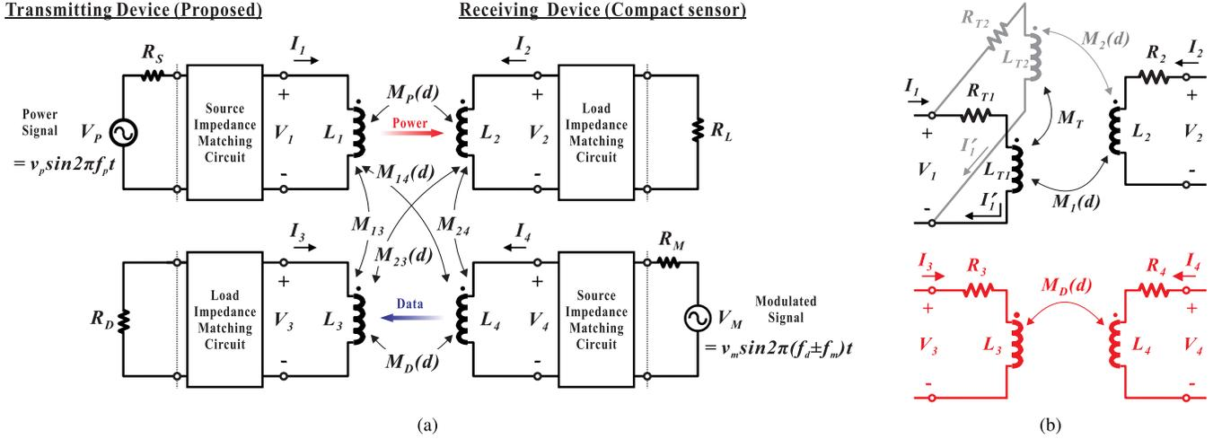
Fig. 4. Overall system configurations. (a) Block diagrams of a longitudinally misalignment-insensitive WPDT system for a loosely coupled compact wireless sensor. (b) Simplified equivalent circuits of proposed loosely coupled transmitting and receiving antenna configurations with a large air gap.
