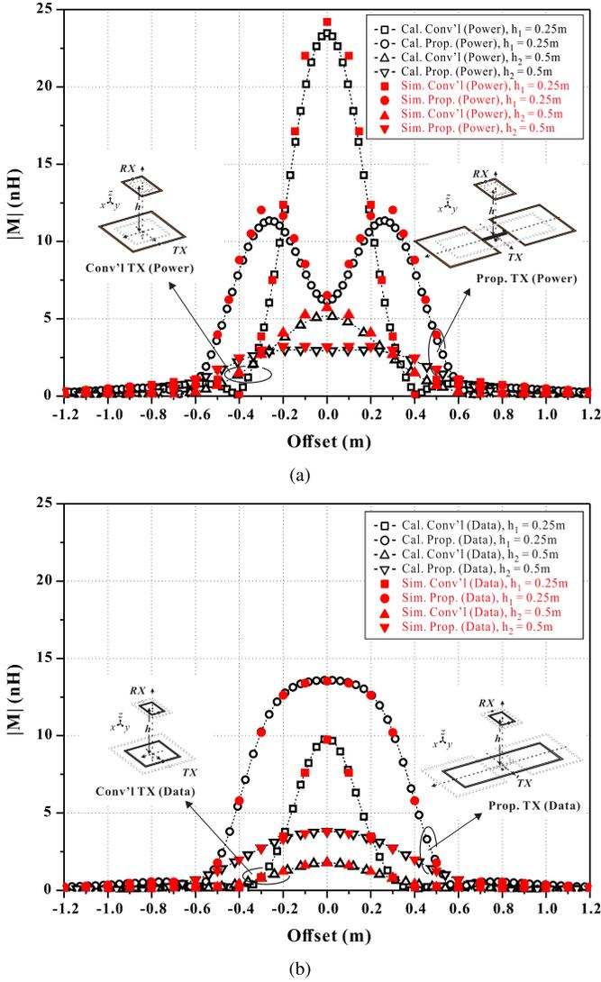
Fig. 6. Calculated and simulated mutual inductances for the conventional and proposed power and data transmitting antennas under a single-turn receiving coil with regard to the air gaps ( $h_1 = 0.25$  m and  $h_2 = 0.5$  m). (a) Downlink power transfer. (b) Uplink data transfer.
