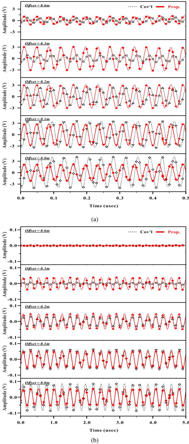
Fig. 15. Signal waveforms between the transmitting and receiving antennas regarding different offsets (0 m ~ 0.6 m) distances at  $h_1 = 0.25$  m. (a) Power transfer link (TX input power: 1 W at 27.1 MHz). (b) Data communications link (TX input power: 1 mW at 4.23 MHz).
