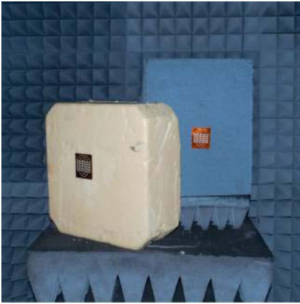
Fig. 12. Target measurement configuration for dual-tag detection demonstration.
