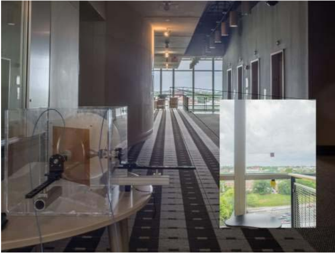
Fig. 15. Measurement configuration at an interrogation range of 30.5 m.
