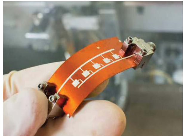
Fig. 2. Inkjet-printed flexible linear antenna array.
