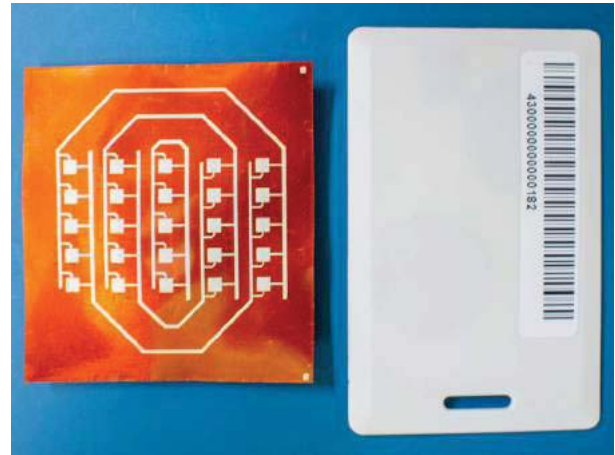
Fig. 5. Inkjet-printed flexible Van-Atta reflectarray prototype, next to a standard “credit card” size RFID tag package.
