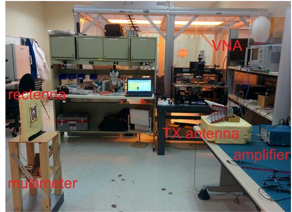
Fig. 21. Test of the rectenna in laboratory: experimental setup.
