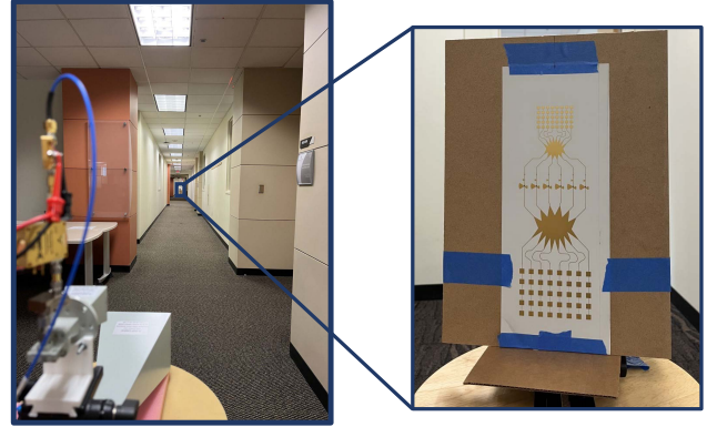
Fig. 10. Harmonic FMCW radar interrogation of the dual Rotman lens-based mmID at 46 m.
